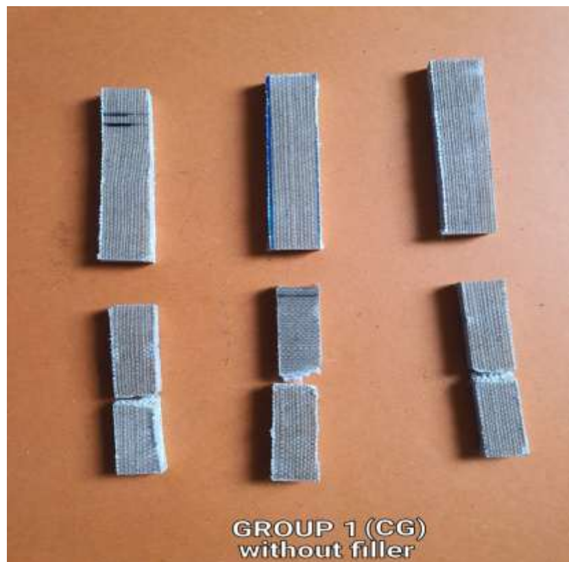
Fig. 2. Specimens without novel \text{Al}_2\text{O}_3 +glass beads before and after Izod impact testing
