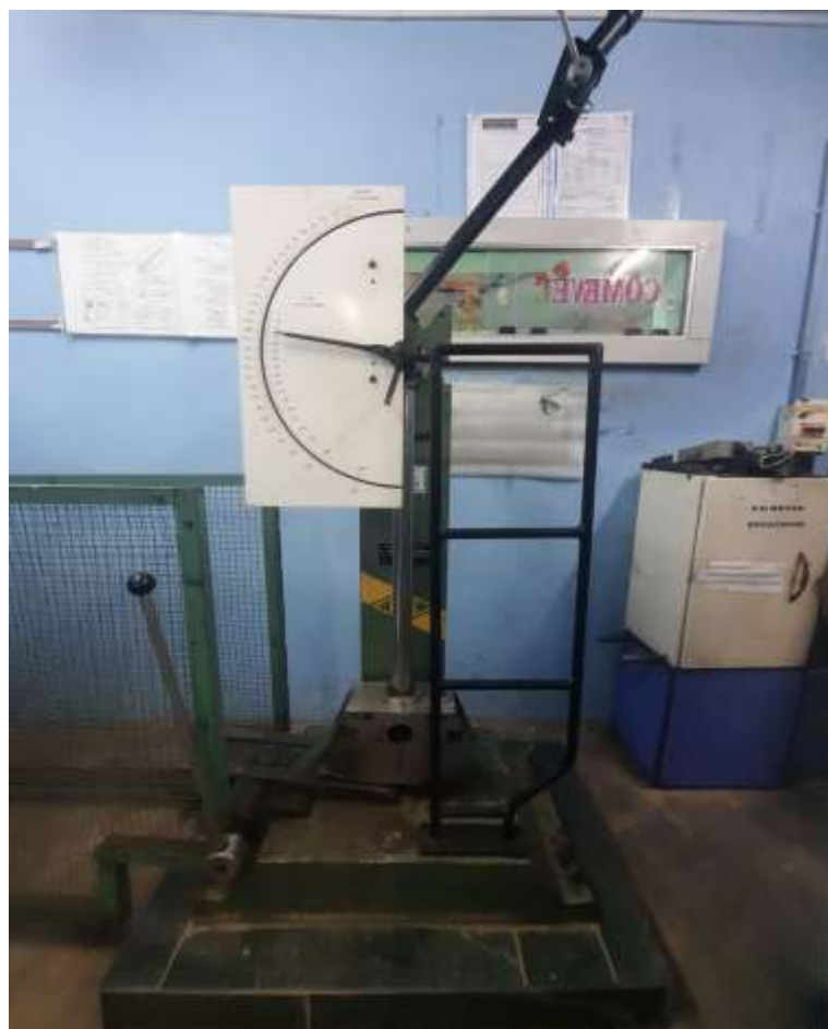
Fig. 4. Impact Testing Machine (IT-30, M/s Fine manufacturing Industries, India) used for Izod impact test
