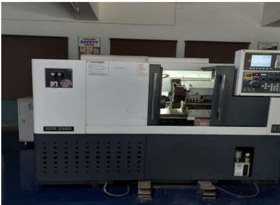
Fig. 1. CNC turning machine center - specifications: swing carriage - 260 mm, maximum turning diameter - 290 mm, maximum turning length - 400/500 mm, swing bed - 500 mm, max spindle speed - 4000 rpm, no of station - 8, chuck size - 200/250.
