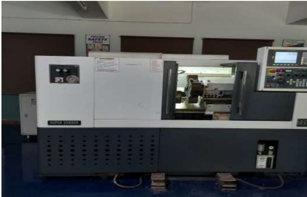
Fig .1. CNC turning machine center - specifications: swing carriage - 260 mm, maximum turning diameter - 290 mm, maximum turning length - 400/500 mm, swing bed - 500 mm, max spindle speed - 4000 rpm, no of station - 8, chuck size - 200/250.
