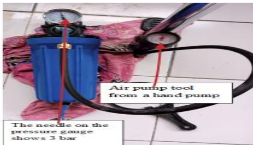
Figure 10. Air filter leakage test
