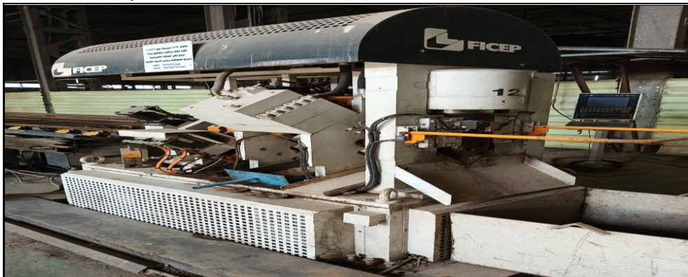
Picture(1) CNC machine programmed to cut, punch and seal metal sections in Al-Samoud Company in Taji District
